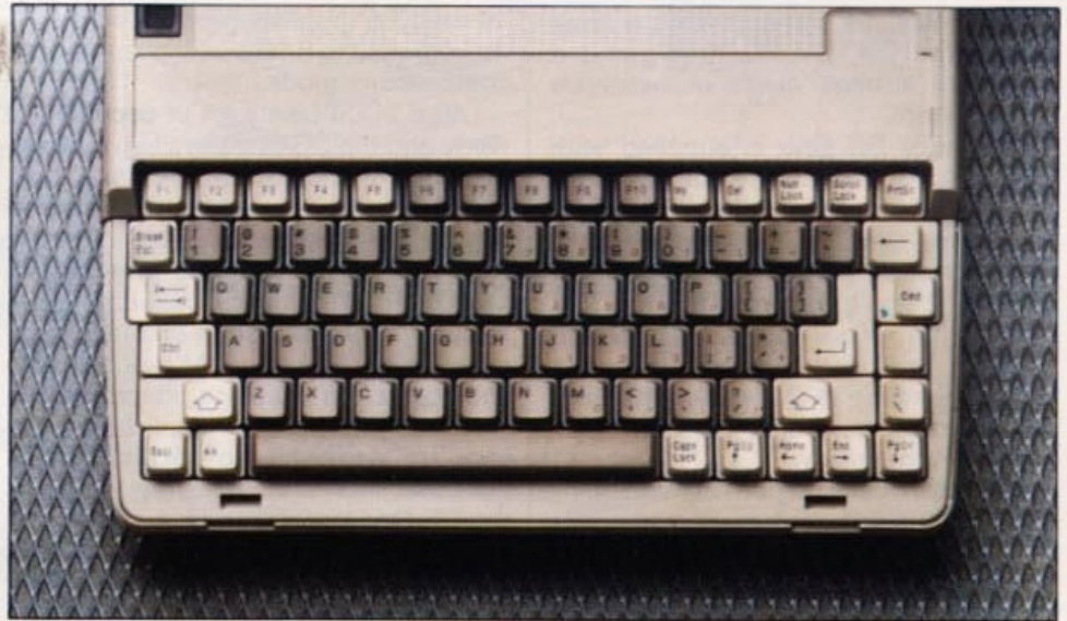
The keyboard is very cramped: 79 keys are squeezed together tightly
